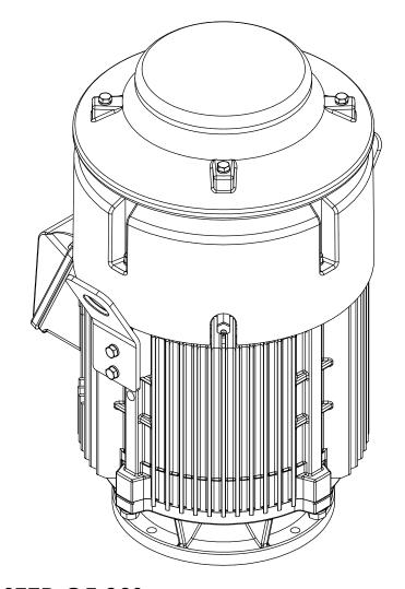
\*\* CONDUIT BOX CAN BE ROTATED IN STEP OF 90°
