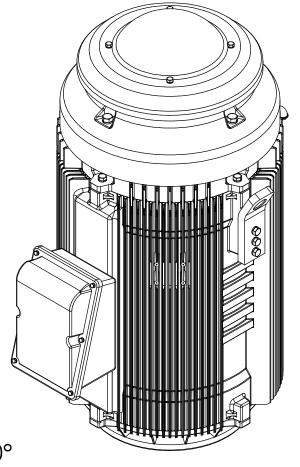
\*\* CONDUIT BOX CAN BE ROTATED IN STEP OF 90°
