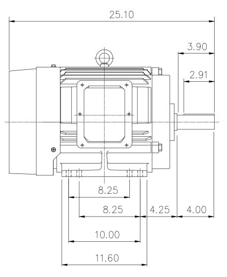
SYN. SPEED OUTPUT POLE VOLT FREQ. (1) DIMENSIONS ARE IN INCHES. CERTIFIED BY (2) APPROXIMATE WEIGHT = 325 lb. (3) DRIVE END BEARING 6310ZZ DR. BY <u>W. D. KUD</u> DIMENSION OPPOSITE DRIVE END BEARING 6208ZZ TATUNG CK, BY L. J. LEE SHEET APP. BY T. M. LIAD (4) INTERNAL VOLUME OF CONDUIT BOX=110.9 CU, IN. DATE NOV. 27. 2008
